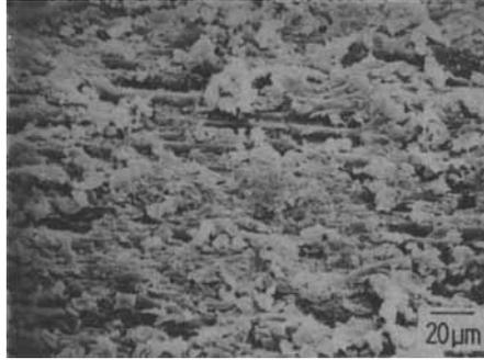
**FIGURE 2** Scanning electron micrograph of abraded/solvent-cleaned APC-2 thermoplastic composite.
